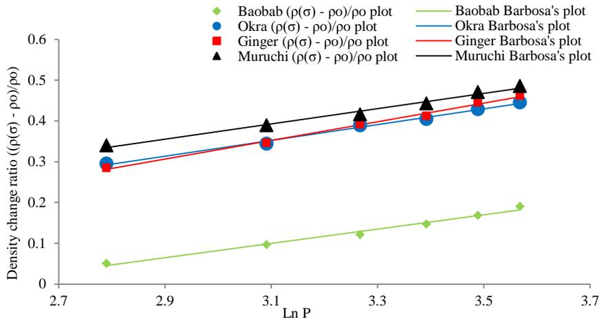
Figure 6: the plots of density change ratio and Barbosa and Co simulation for baobab, okra, ginger and muruchi powders
