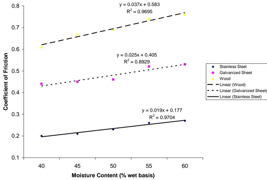
**Figure 1: Coefficient of Friction of TMS 30572 Cassava Cultivar**
