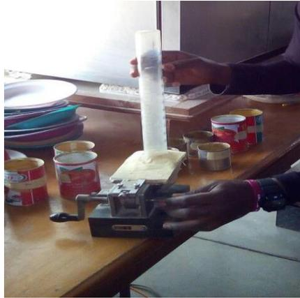
Plate 1: Tapping apparatus
