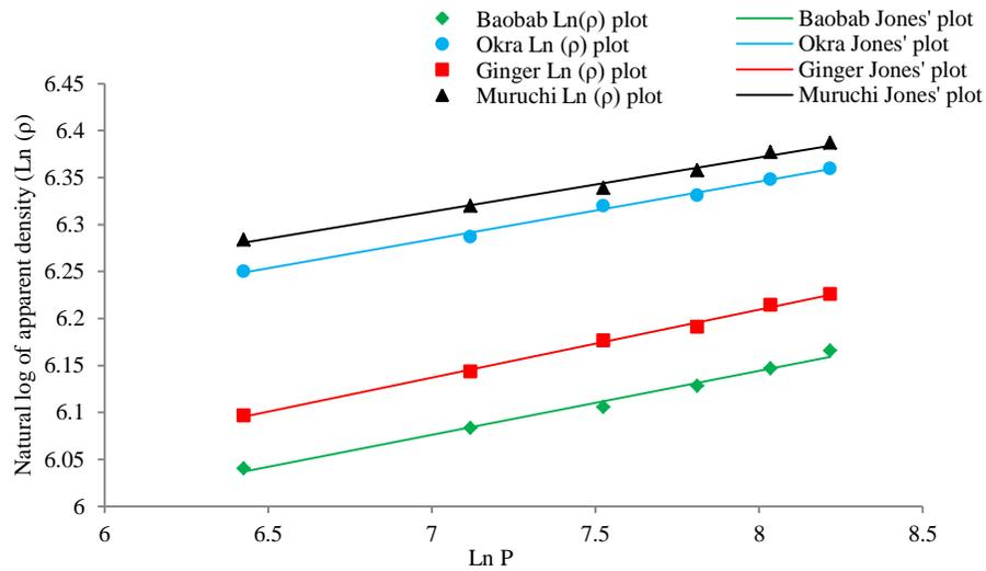
Figure 5: the plots of natural log of apparent density at applied lpressure and Jones' simulation for baobab, okra, ginger and muruchi powders
