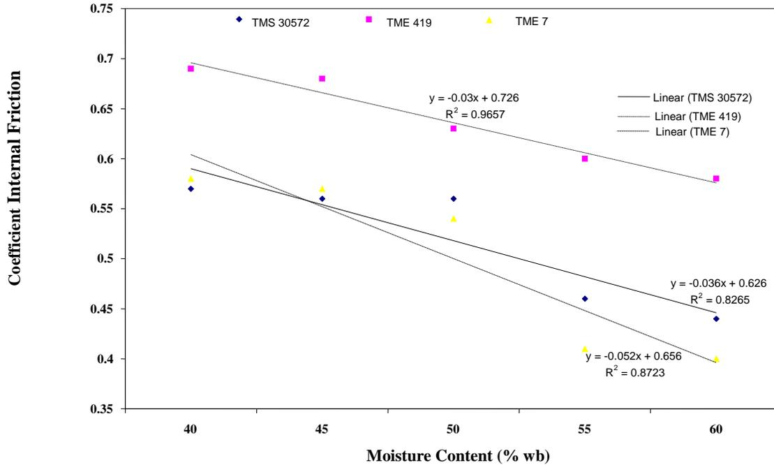
**Fig 4: Coefficient of Internal Friction of Cassava**
