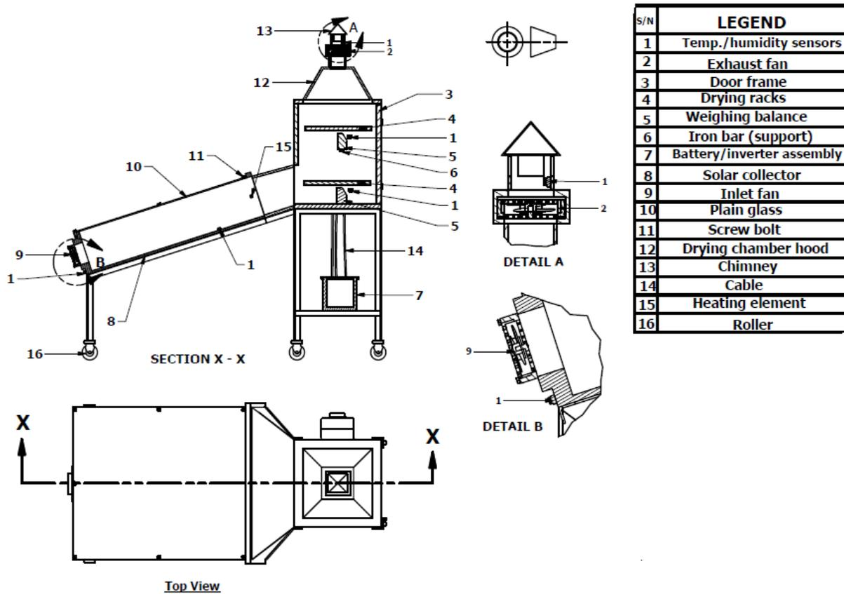
Figure3: Sectional view of the hybrid dryer.
