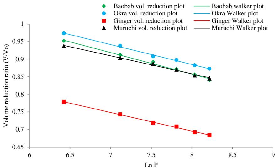
Figure 4: the plots of volume reduction ratio and Walker's simulation for baobab, okra, ginger and muruchi powders
